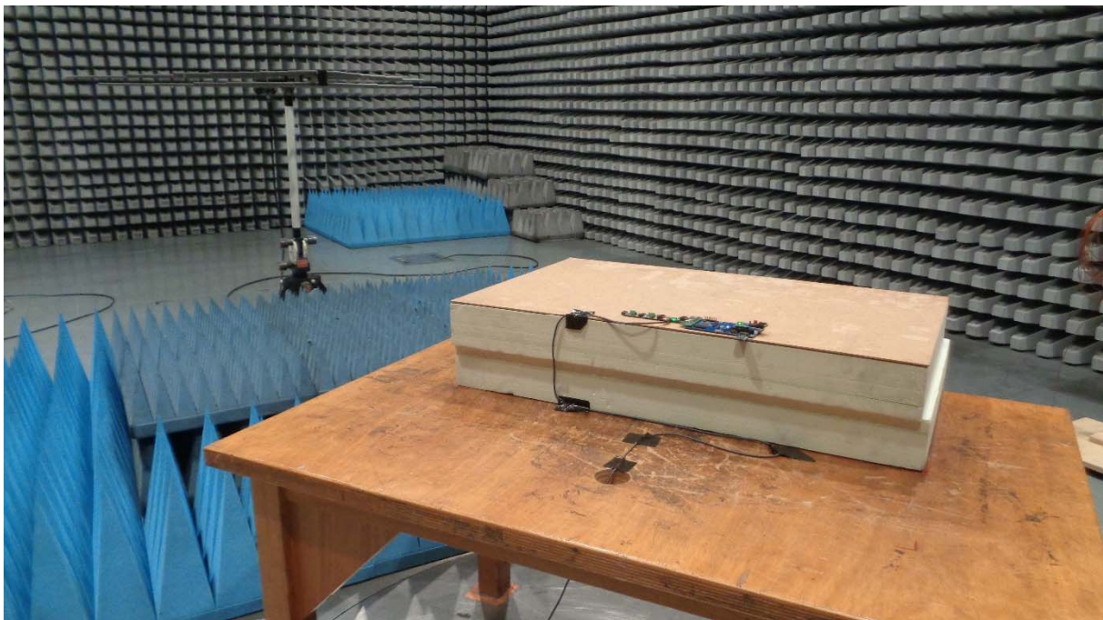
Fig. 5.2.2: Real radiated immunity measurement setup 80 MHz to 1 GHz.
